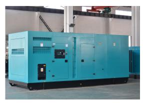
Dimension:5800\*2300\*2500mm Weight:11500kg Fuel Tank Capacity:1200L The **control panel** is an Digital Control Module suitable for a wide variety of single, diesel or gas, gen-set applications.
