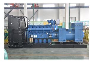
Dimension:6830\*2745\*3100mm Weight:17500kg Fuel Tank Capacity:1000-3000L The **control panel** is an Digital Control Module suitable for a wide variety of single, diesel or gas, gen-set applications.
