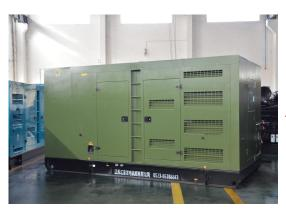
Dimension:4300\*2000\*2250mm Weight:5500kg Fuel Tank Capacity:850L
