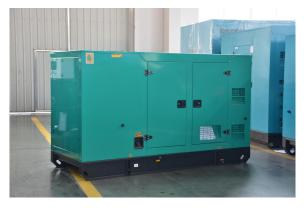
Dimension:3000\*1100\*1700mm Weight:2300kg Fuel Tank:280L The **control panel** is an Digital Control Module suitable for a wide variety of single, diesel or gas, gen-set applications.
