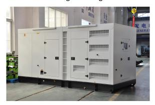
Dimension:5200\*2100\*2400mm Weight:10100kg Fuel Tank Capacity:1000L
