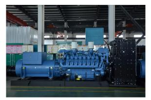
Dimension:8230\*2600\*2700mm Weight:20000kg Fuel Tank Capacity:1000-3000L The **control panel** is an Digital Control Module suitable for a wide variety of single, diesel or gas, gen-set applications.
