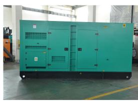
Dimension:4300\*2000\*2250mm Weight:4600kg Fuel Tank Capacity:850L The **control panel** is an Digital Control Module suitable for a wide variety of single, diesel or gas, gen-set applications.
