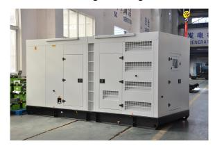
Dimension:4700\*2100\*2400mm Weight:8000kg Fuel Tank Capacity:1000L
