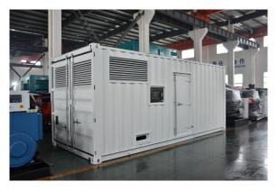
Dimension:6000\*2400\*2900mm Weight:10300kg Fuel Tank Capacity:1000-3000L
