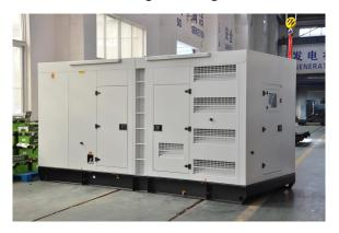
Dimension:4700\*2100\*2400mm Weight:6200kg Fuel Tank Capacity:1000L
