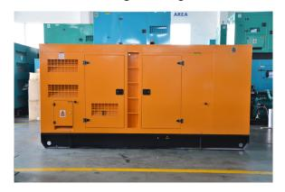
Dimension:4000\*1700\*2000mm Weight:5200kg Fuel Tank Capacity:680L
